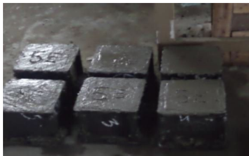
Fig.1 Concrete cubes replaced with coconut and sea shells aggregate
